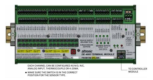
\*Be sure to note the changes to the DIP switch settings when replacing a Terminal Module. Digital NO, 4-20mA and Unused Inputs have different settings than the legacy Terminal Module.
